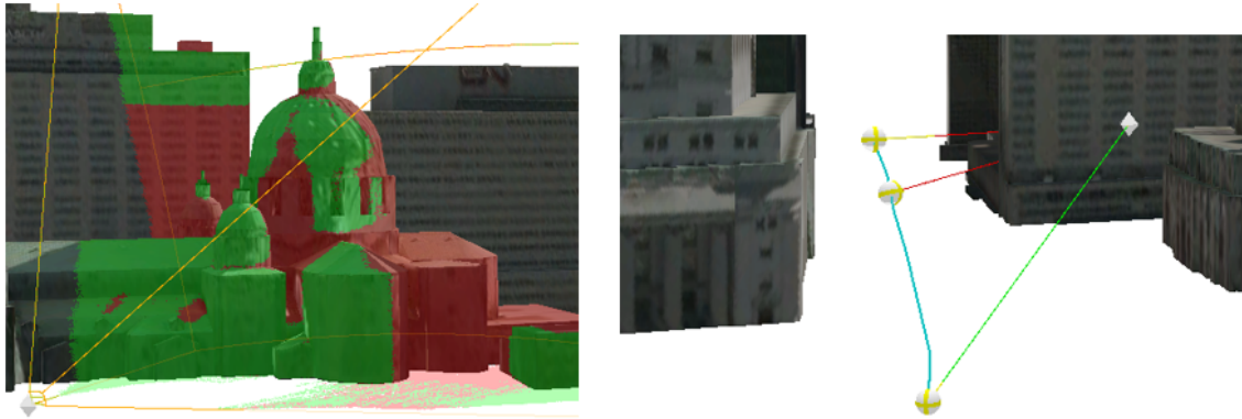
Figure 13.5. Interactive 3D analysis tools: Viewshed (on the left) and Line Of Sight (on the right).
