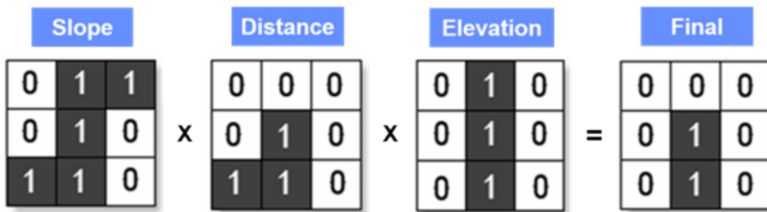
Figure 7.10. For each input surface, a 1 indicates that a cell is suitable. The final result reveals that only two cells are suitable based on the criteria; all other cells (for example, cells with a value of 0) are considered unsuitable.
