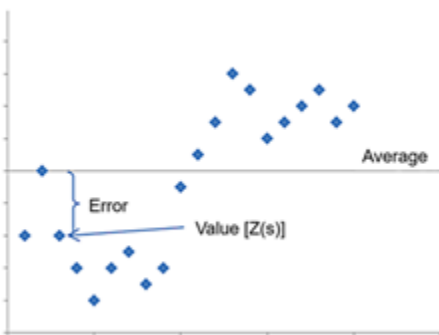
Figure 12.5. All these blue points represent a sample location that includes a temperature value. Thus, you can calculate a mean, which is a statistic. Deterministic methods ignore even basic statistics, such as the mean.
