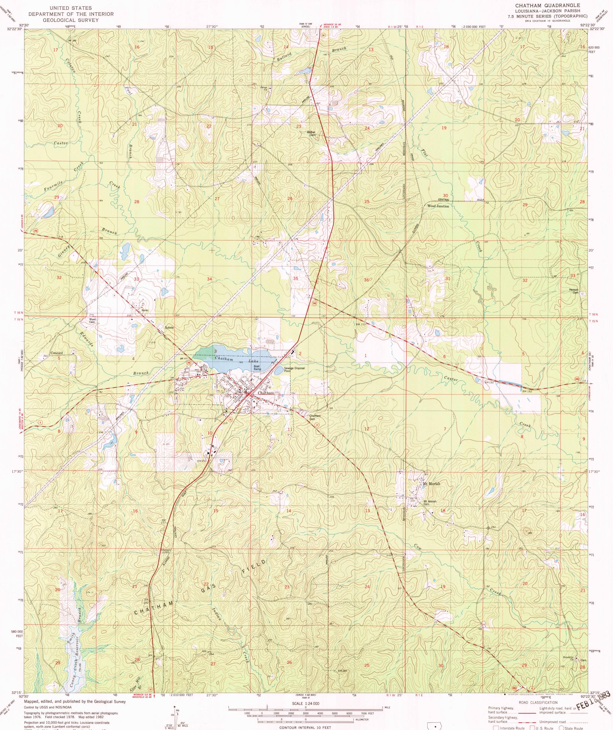
system, north zone (Lambert conformal conic) 1000-meter Universal Transverse Mercator grid, zone 15 1927 North American Datum To place on the predicted North American Datum 1983 move the projection lines 13 meters south and 14 meters east as shown by dashed corner ticks
