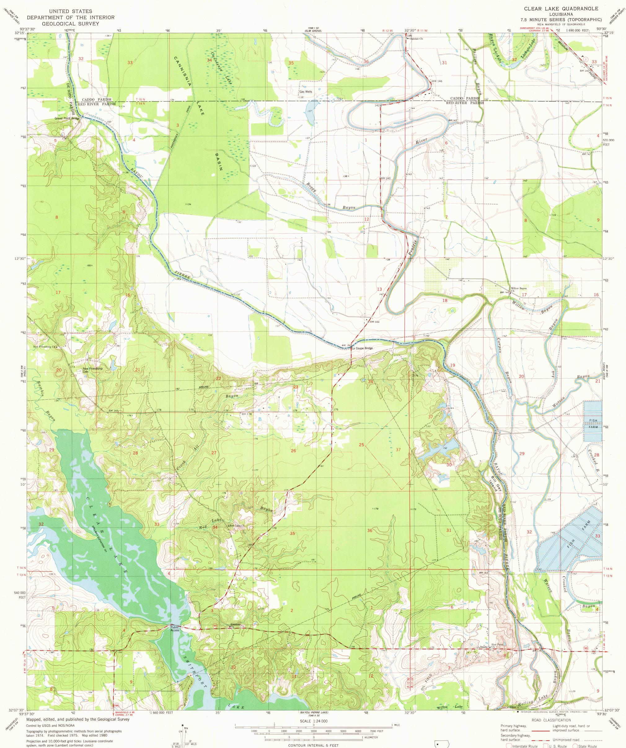
system, north zone (Lambert conformal conic) 1000-meter Universal Transverse Mercator grid, zone 15 1927 North American Datum To place on the predicted North American Datum 1983 move the projection lines 13 meters south and 17 meters east as shown by dashed corner ticks
