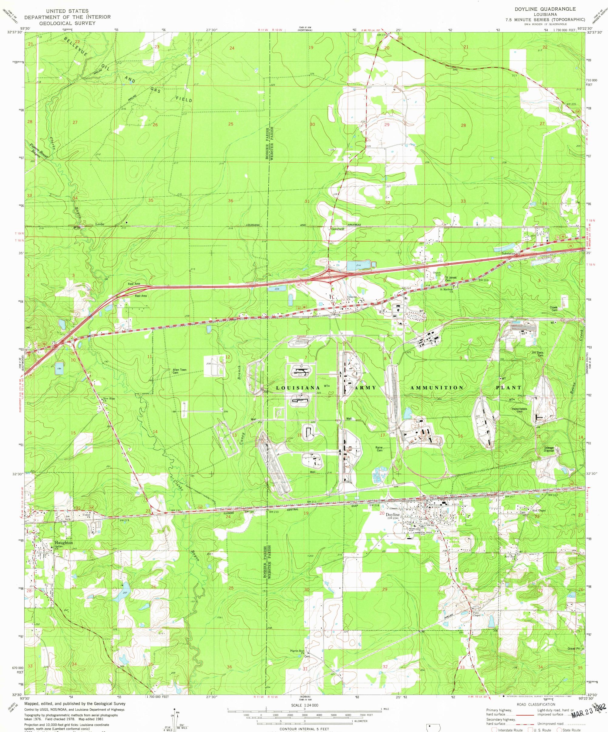
system, north zone (Lambert conformal conic) 1000-meter Universal Transverse Mercator grid, zone 15 1927 North American Datum To place on the predicted North American Datum 1983 move the projection lines 12 meters south and 17 meters east as shown by dashed corner ticks
