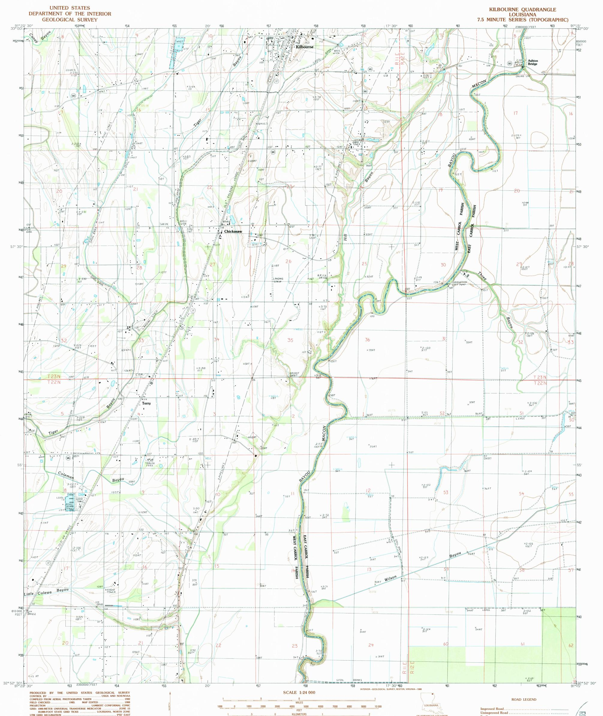
1988 MAGNETIC NORTH DECLINATION... 3°00' EAST To place on the predicted North American Datum of 1983, move the projection lines as shown by dashed corner ticks (12 meters south and 11 meters east) There may be private inholdings within the boundaries of any Federal and State reservations shown on this map No distinction made between houses, barns, and other buildings
