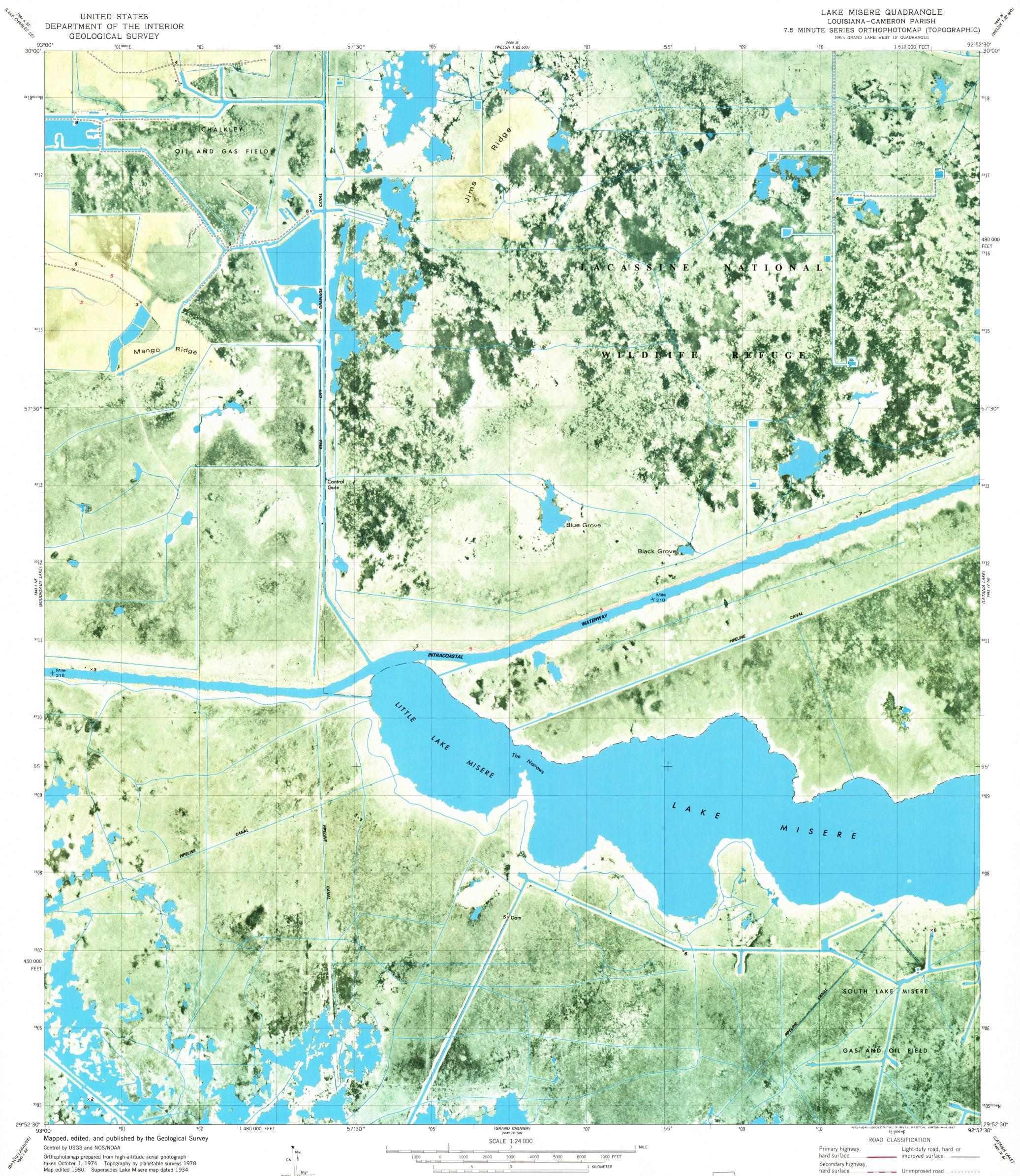
Projection and 10,000-foot grid ticks: Louisiana coordinate system, south zone (Lambert conformal conic) 1000-meter Universal Transverse Mercator grid, zone 15 1927 North American Datum To place on the predicted North American Datum 1983 move the projection lines 19 meters south and 15 meters east as shown by dashed corner ticks
