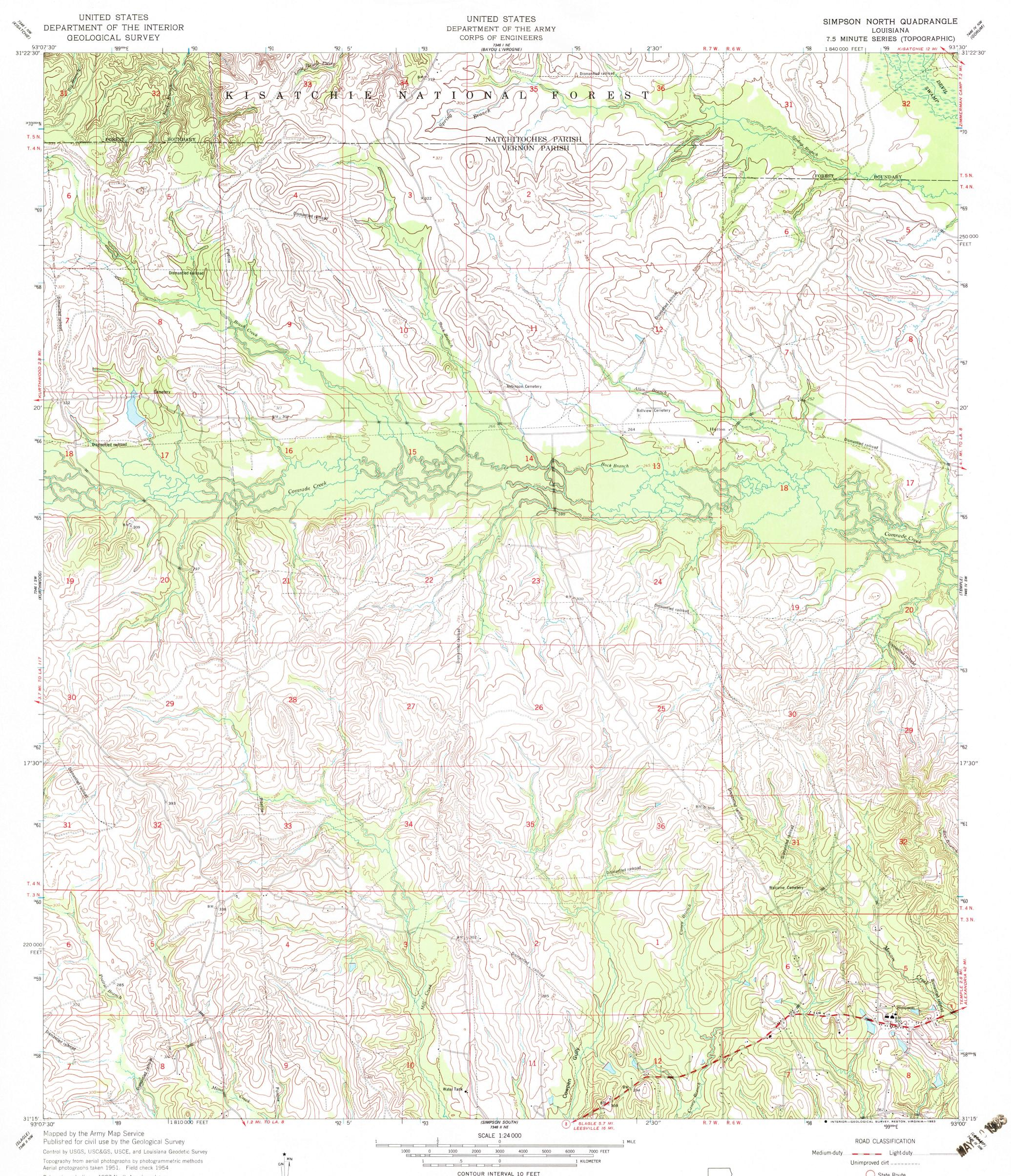
Polyconic projection. 1927 North American datum 10,000-foot grid based on Louisiana coordinate system, north zone 1000-meter Universal Transverse Mercator grid ticks, zone 15, shown in blue To place on the predicted North American Datum 1983 move the projection lines 16 meters south and 15 meters east as shown by dashed corner ticks
