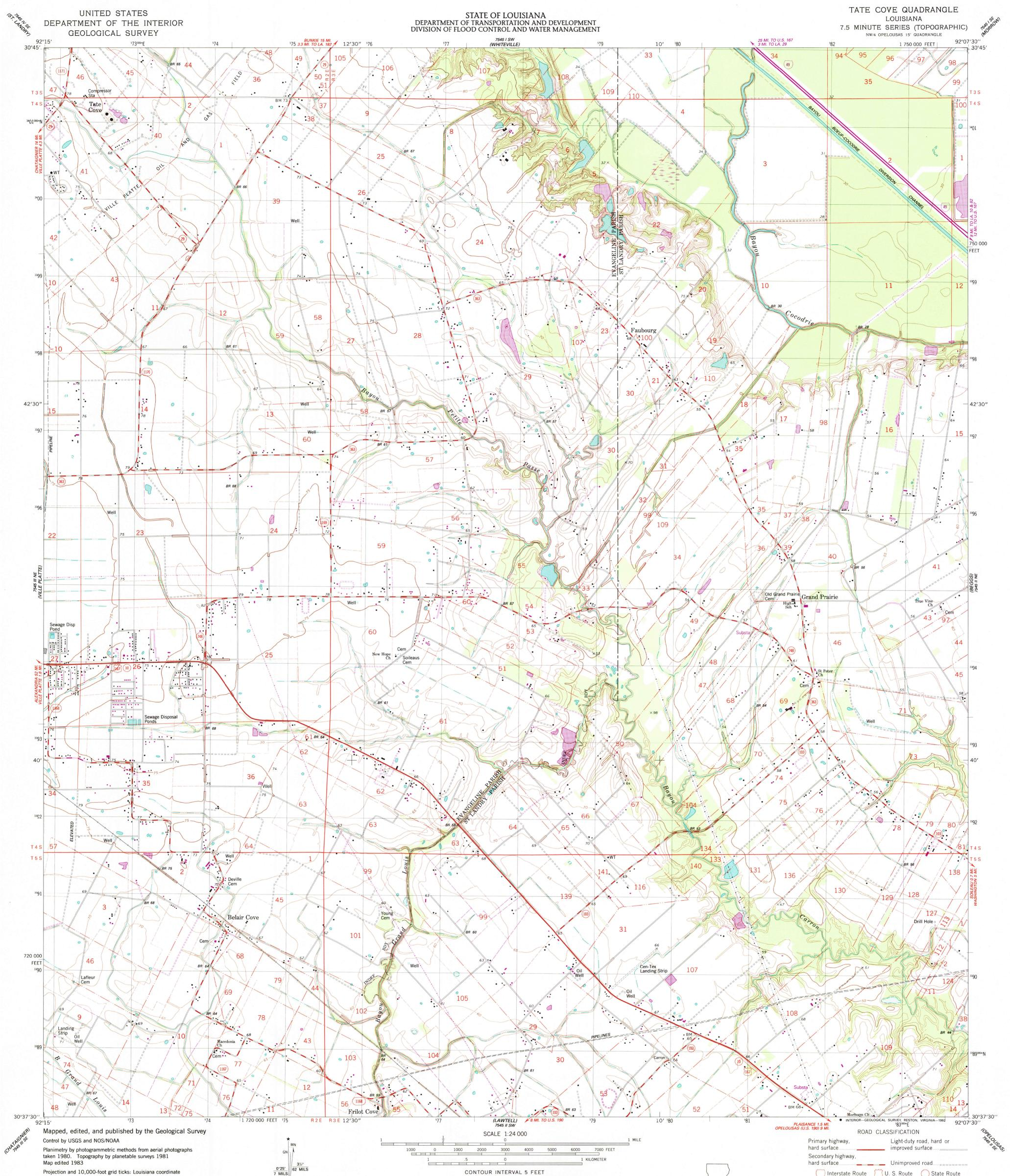
Projection and 10,000-foot grid ticks: Louisiana coordinate system, south zone (Lambert conformal conic) 1000-meter Universal Transverse Mercator grid, zone 15 1927 North American Datum To place on the predicted North American Datum 1983, move the projection lines 17 meters south and 13 meters east as shown by dashed corner ticks
